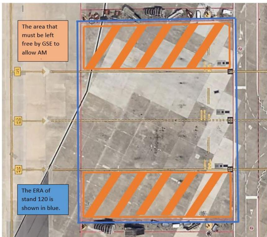
**Do not park** in the area marked with orange zebra stripes, which is reserved for GSE vehicles used to set up the stand while awaiting the arrival of the AM.
